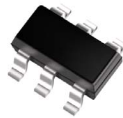
Figure 2. Package Type 6-lead SOT23
